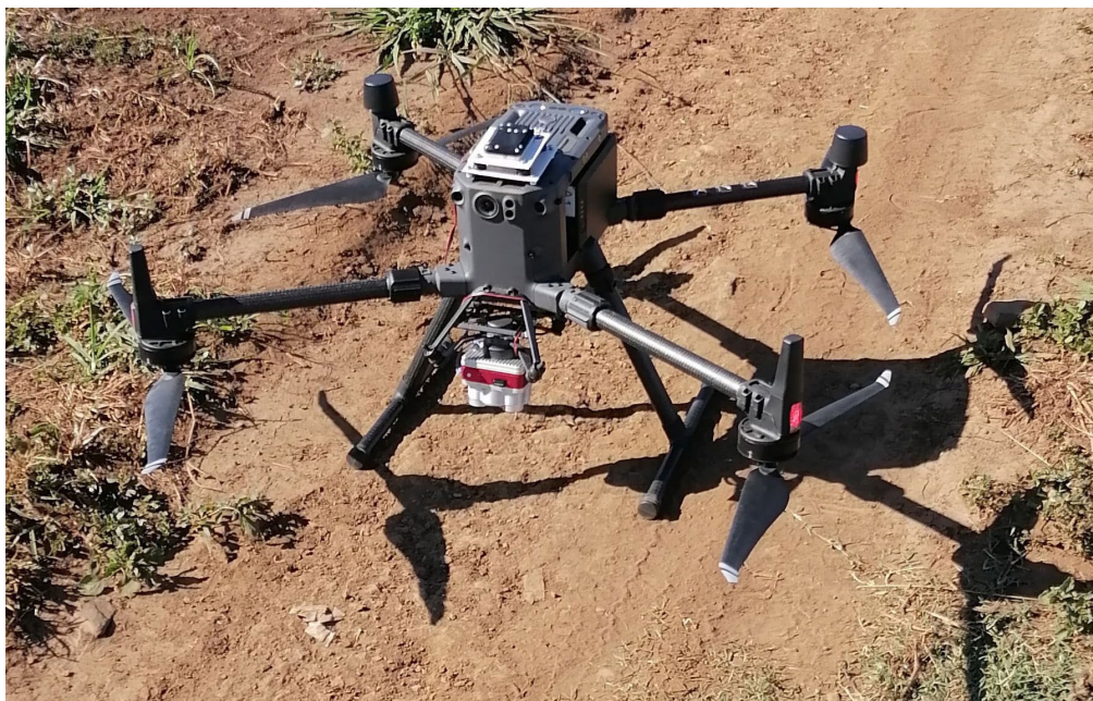
Plate 1: DJI Matrice 300 series drone with mounted MicaSense Altum camera used for imagery acquisition over the growing season
